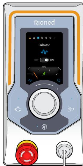
The diesel engine is being preheated or the high-pressure pump is running dry or the oil level is too low
