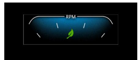
The tachometer status is always displayed. This status depends on where you are in the menu. The pointer indicates the current speed in revolutions per minute (1 line is 1000 rpm).
