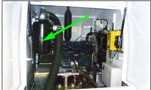
**9.5 Vacuum blow off container** Drain the container regularly.
