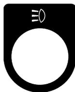
By means of switch
