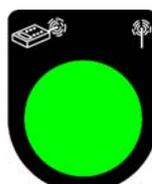
Signal lamp “Radio remote control” on
