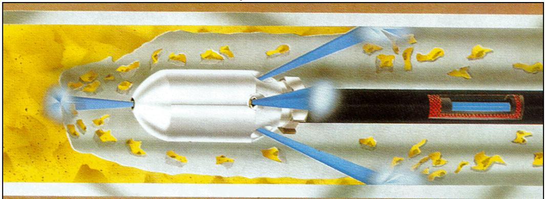
7. Check that the water drains away. When the blockage has been cleared, continue to flush for a while. At the same time wind the hose up slowly.
