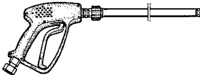
b Unclogging of a drain: jet nozzle.
