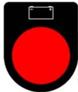
Signal lamp "Charging" (*Burns if there is no charge to the battery.*)
