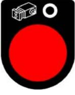
(HP pump off) or “HP off”
