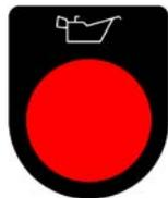
Signal lamp "Oil pressure" (*Burns if there is not enough oil in the engine.*)
