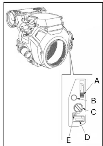
9. Warm up the engine for 2 or 3 minutes. If the choke knob was pulled to the CLOSED position to start the engine, gradually push it to the OPEN position as the engine warms up.
